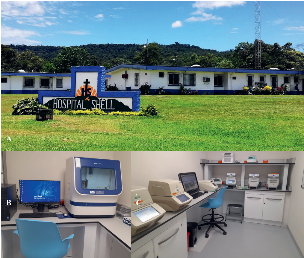
Figure 4. A) Shell hospital included the majority of the participants from the Amazon. B) The sequencer used to differentiate Leishmania species at the research laboratory of the Universidad de Las Americas in Quito. C) The thermocyclers used for qPCR to detect Leishmania DNA from samples dried on filter paper at the research laboratory of the Universidad de las Americas in Quito. Image A: Copyright © 2022 Hospital Shell, All rights reserved., Image B and C: Copyright © 2023 Manuel Calvopiña, All rights reserved. All images were used with the permission of the copyright holders.
